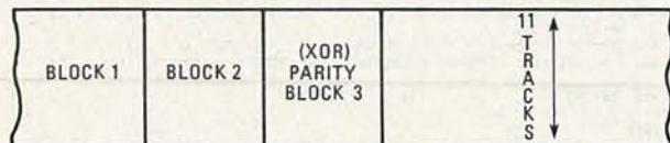
Fig. 2—THE PC/T APPROACH uses a single head to write data to tape in two 4K blocks. Using the same data as in the first two blocks, a third parity block is constructed by performing an exclusive or operation. In this way, should data be lost, it can be more-easily reconstructed during an error recovery pass. This does increase system overhead.
