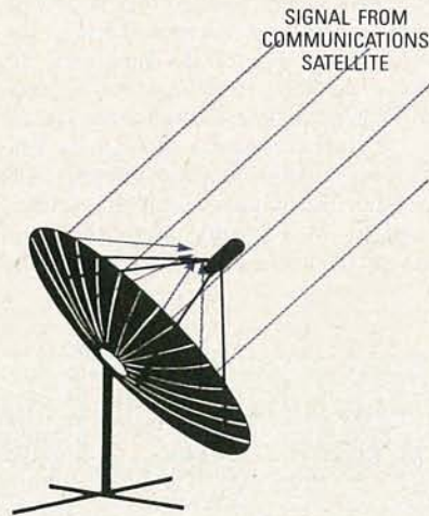
FIG. 3—BECAUSE THEY HAVE PROPERTIES similar to those of light, microwave signals can be collected and focused on an antenna element by a metallic surfaced reflector. That property is the basis of the satellite dish. The satellite dish is the radio equivalent of the optical reflecting telescope.
