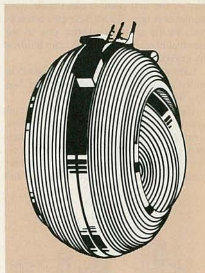
FIG. 8—A VARIO-COUPLER, or variometer, consisted of two coils mounted in such a way that one could be rotated within the other.
