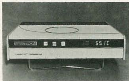
FIG. 17—LUXTRON'S FLUOROPTIC THERMOMETER has both analog and digital outputs for peripheral devices.
