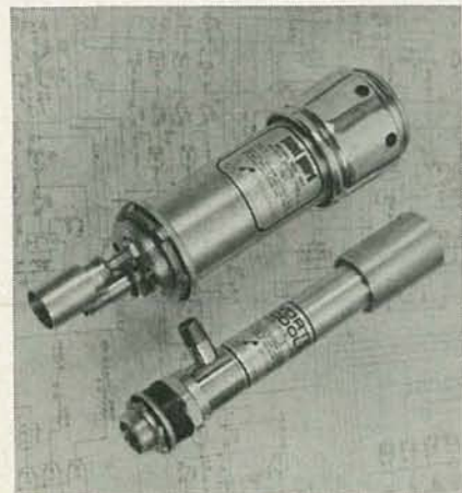
FIG. 27—A THERMOSTAT may be an integral part of a vortex tube.
