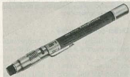
FIG. 15—THIS "TEMPILSTIK"™ changes color at 121°C.
