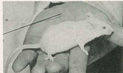
FIG. 19—A FLUOROPTIC PROBE can also pass directly into a biological research specimen.
