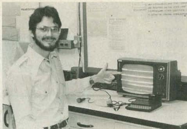
FIG. 1--AUTHOR POINTS TO SCREEN as computer runs in the "speaking" mode. TV lines flicker according to outputted sound.
