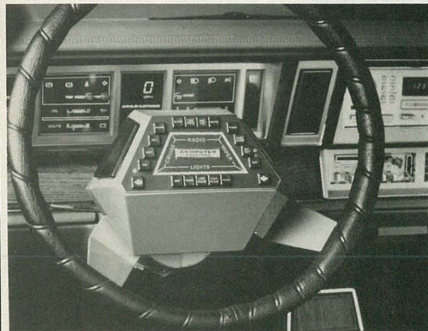
FIG. 6—IN THE CHRYSLER STEALTH concept car, many controls have been relocated to the steering wheel. In that vehicle, the traditional wiring harness has been replaced with a multiplexed wiring scheme.
