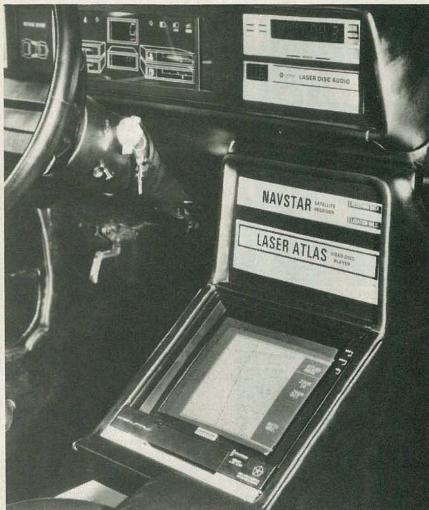
FIG. 5—CHRYSLER'S CLASS system uses a satellite receiver to obtain navigational information from a system of orbiting satellites.
