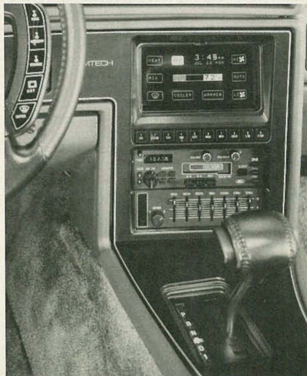
FIG. 1—CRT IN FORD 1985 Mark VII Comtech displays driver information and permits manipulation of such items as climate control simply by touching the screen.
