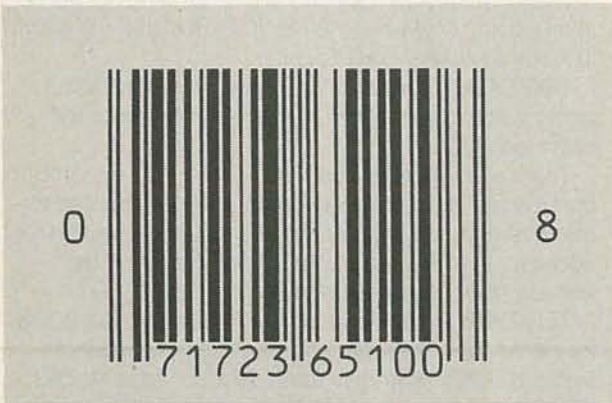
FIG. 1—UNIVERSAL PRODUCT CODES are one method of data input. Special readers interpret the strip and convert the information into useable data for a computer.
