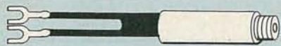
FIG. 2—A 75-OHM-TO-300-OHM matching transformer or adaptor is used to connect a coaxial cable to the antenna input terminals at the back of a TV set.
