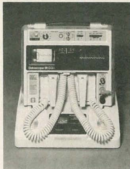
FIG. 4—A DEFIBRILLATOR uses electrical shock to restore a heartbeat to normal.
