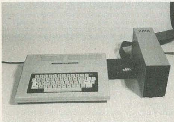
THE COCO WITH THE DISK DRIVE WHEN COMPLETED. If you want two drives, simply install a second connector on the ribbon.
