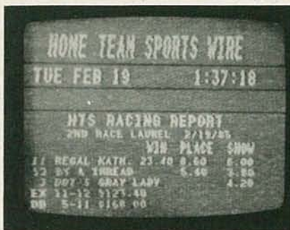
NOISE IN THE VIDEO results from an insufficient carrier-to-noise ratio, which is a function of antenna gain (size), LNA noise-temperature, and receiver design. This is the reception quality afforded by an 8-foot dish in a weak signal area.
