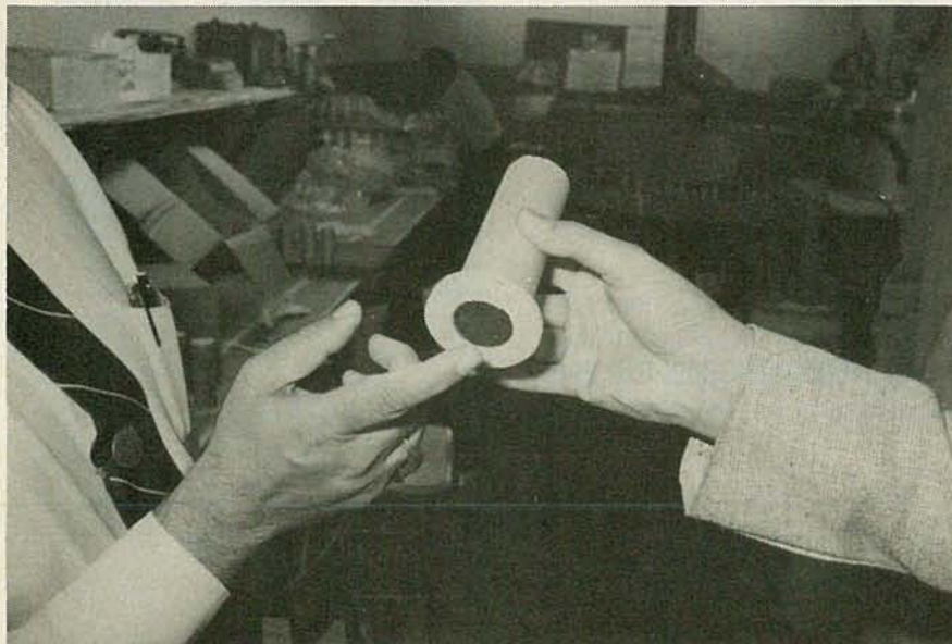
NEW MAGNESIUM BATTERY features an "inside-out" construction. The positive element serves as both the center electrode and the battery can.
