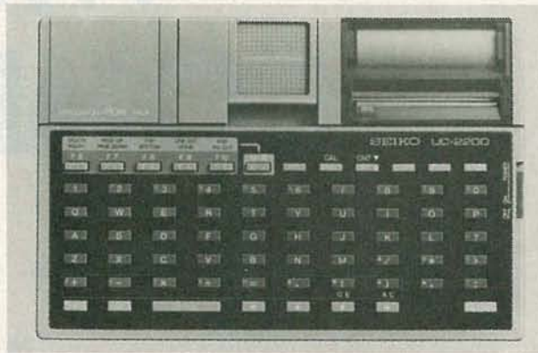
THE UC-2200 CONTROLLER turns the display module into an 8-bit micro-computer. The controller is shown here with an application ROM pack in place.
