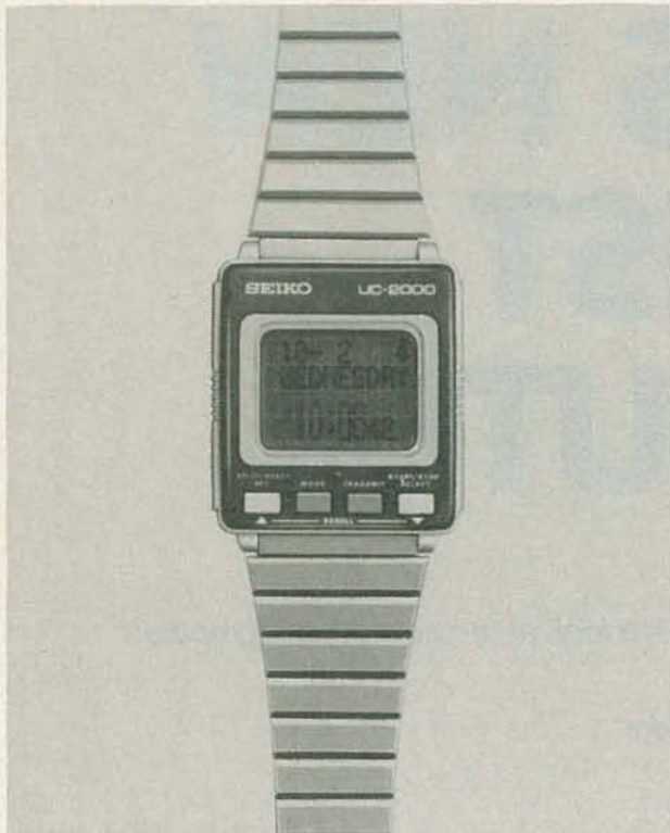
THIS IS NOT a wrist watch! It is the display module for the Seiko Datagraph computer.
