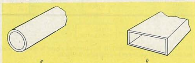
FIG. 3—A WAVEGUIDE may be cylindrical, as shown in a, or rectangular, as shown in b.
