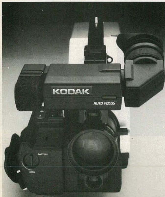
THE KODAVISION 2400 "CAMCORDER" combines video camera and recorder, with a cassette little larger than an audio tape cassette. Extremely portable and maneuverable, the 8-mm unit weighs only a little over 5 pounds.
