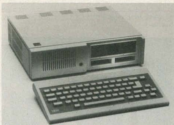
FIG. 2—THE IBM PCjr. The version shown here features a single disk drive, two cartridge slots, and a cordless keyboard.
