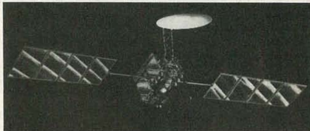
ARTIST'S REPRESENTATION OF THE HIGH-POWERED direct-broadcasting satellite that STC plans to use in 1986 to beam programming to both the Eastern and Central time zones. Each of the two satellites will carry three channels and will transmit 200-watt signals.
