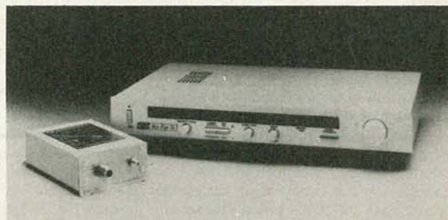
FIG. 1—SATELLITE TV RECEIVER. Features of this unit (KLM Sky Eye V11X) include variable speed scanning for fast scanning of the satellites or frame-by-frame viewing of each of the 24 transponders of a satellite. Note that this receiver uses an external downconverter, shown beside it.
