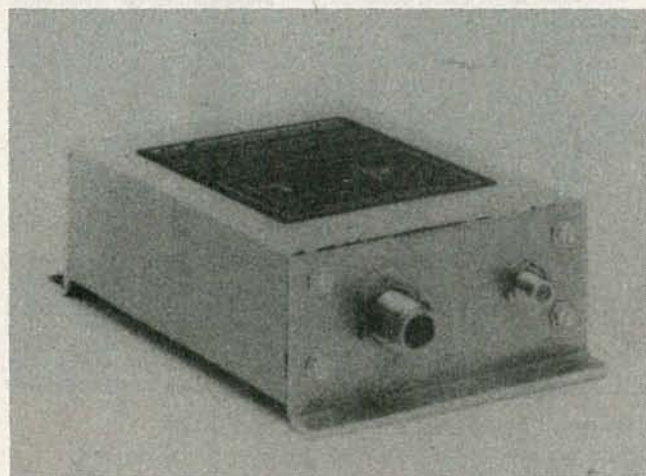
A DOWNCONVERTER IS USED TO convert the high-frequency downlink signals to ones with a lower frequency. Doing that allows standard coax cable to be used.
