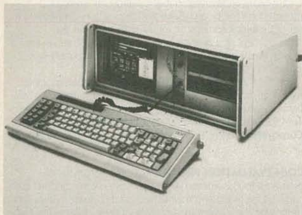
FIG. 1—THE NEW IBM PORTABLE personal computer features 256K of user memory and a single disk drive.
