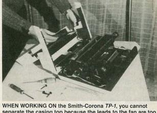
separate the casing top because the leads to the fan are too short.
