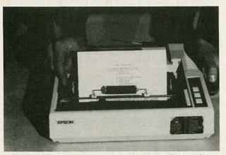
A SINGLE SHEET being printed by the MX-80. Be certain the pin-feed mechanisms are against the sides of the paper it feeds straight.
