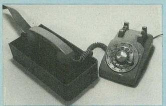
AN ACCOUSTIC-COUPLED modem has rubberized cups into which the telephone handset seats.
