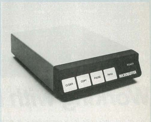
PRINTER BUFFERS like the Microbuffer from Practical Peripherals free the computer for other tasks during printing.
