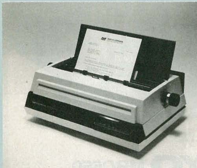
THE SMITH-CORONA TP-1 was one of the first low-cost, bidirectional daisywheel printers for personal computer use.
