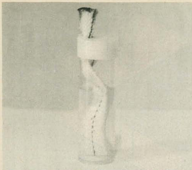
FIG. 6—THE SEEDER USED in our model was made from a coin tube.
