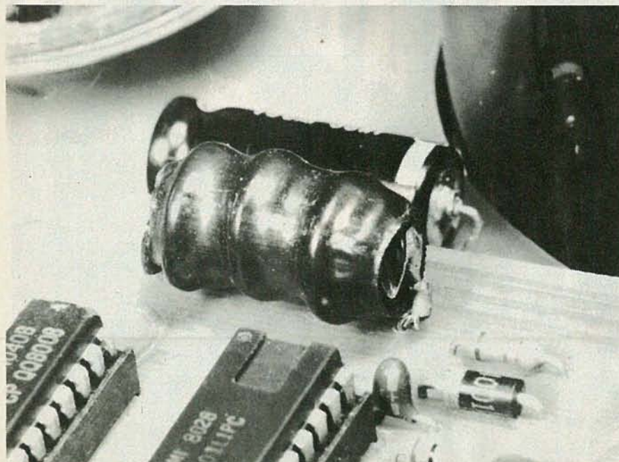
FIG. 18—BATTERIES B9-B11 should be button-cell types with solder lugs. Those batteries can then be soldered together, covered with heat-shrink tubing, and mounted directly on board 1 as shown.
