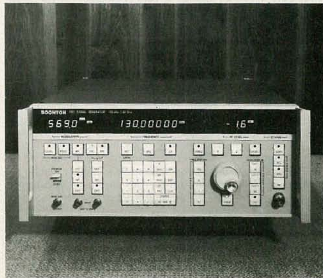
IF YOU'RE SERVICING CELLULAR RADIO equipment, a programmable RF signal generator like the Boonton Electronics model 1021 is what you need. The special feature is that it covers the requirements for high-speed testing of cellular receivers.
