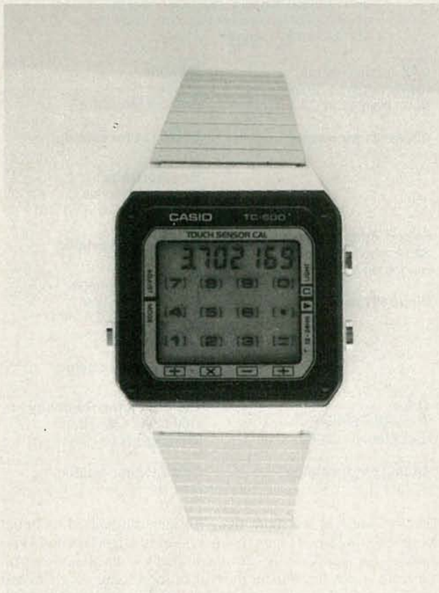
INSTEAD OF KEYS , this calculator/wristwatch from Casio uses a touch sensitive watch face.
