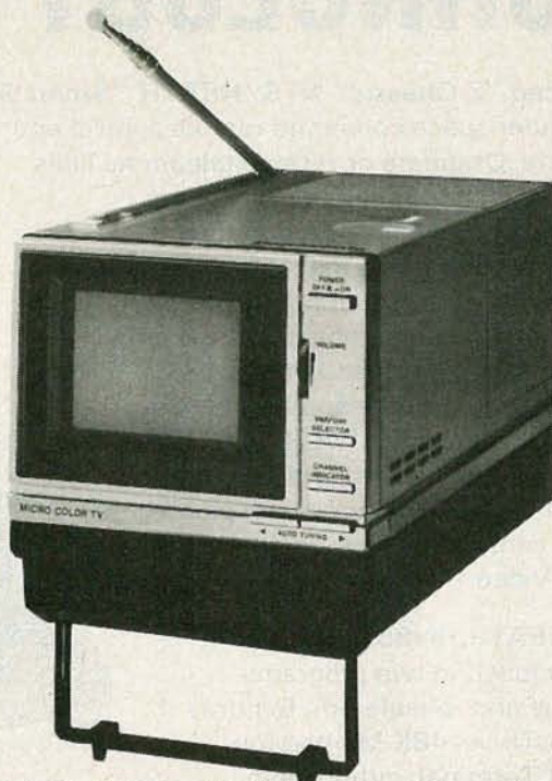
THIS SMALL COLOR PORTABLE from Panasonic has no channel selector dial. Instead, it features an electronic auto-search tuner.
