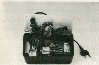
FIG. 2—THE PROJECT IS HOUSED in a small project box with an aluminum front panel. Note the lead to the recorder at the right; it was taken from a defective microphone (see text).
