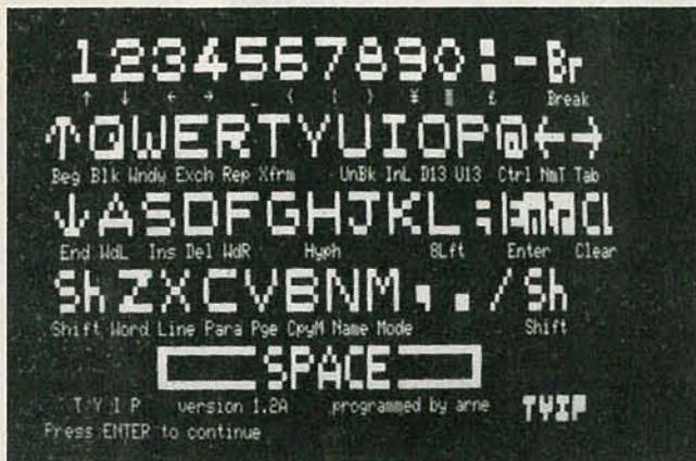
TYPITALL'S HELP SCREEN shows you a representation of the keyboard that shows control and function keys and special characters.
