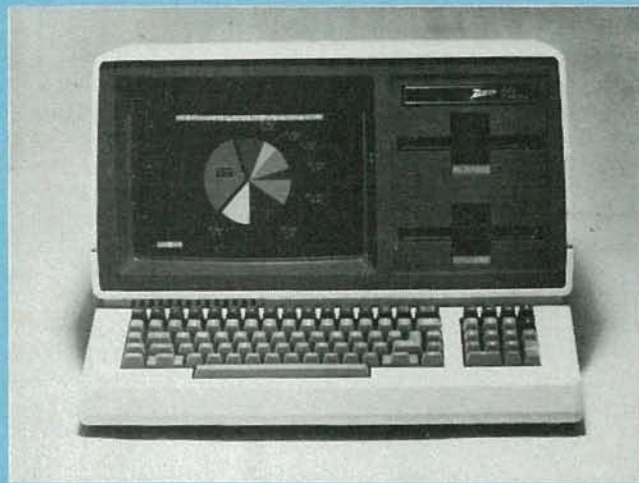
THE ALL-IN-ONE version of Zenith's 8/16-bit computer system, the Z-100 has a non-glare green CRT and two 320K 5¼-inch drives.
