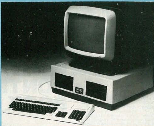
THE BASIS 108 from Basis, Inc. is a dual microprocessor (Z80A/6502) system that runs CP/M and an Apple-compatible DOS.
