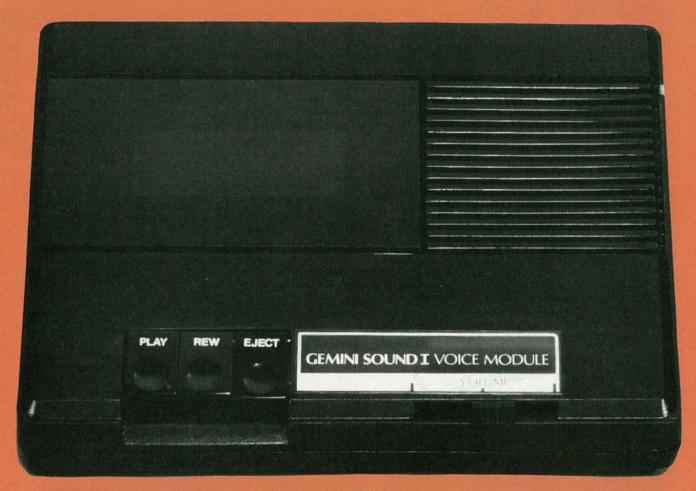
COLECO ADDS VOICE to the Atari 2600 with the Gemini madule that uses special cartridges & tapes.
