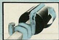
View of wire at end of bit being wrapped on post.
