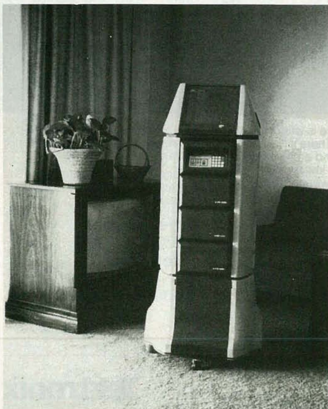
A FORMIDABLE SENTRY, THE ROBOT security monitor stands guard over the home. For that purpose it is equipped with microwave, passive infrared, and audio discrimination detectors. The robot is made by Robotics International Corp. of Jackson, MI.
