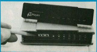
FIG 7—The SMARTMODEM'S OPERATING PARAMETERS can be set from the keyboard or through the use of this DIP switch; the switch is concealed behind the front panel of the device.
