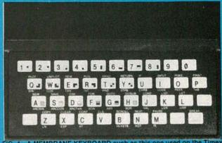
FIG. 4—A MEMBRANE KEYBOARD such as this one used on the Timex/ Sinclair 1000 (Sinclair ZX81) has character, graphics, and BASIC key functions imprinted directly on the membrane—there are no "real" typewriter keys.
