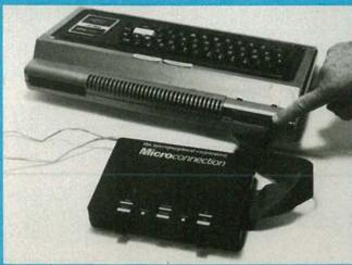
FIG. 3—THIS SPECIAL MODEL of the *Microconnection*, the model *UM1* from the Microperipheral Corporation, works with the Radio Shack *TRS-80 Model I* and eliminates the need for the RS-232 expansion interface.
