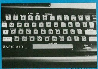
CLEAR PLASTIC TEMPLATE with overprinting for BASIC Aid fits over Color Computer's keyboard. Now, single-key BASIC commands are easy.
