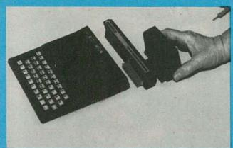
FIG. 2—ADD-ON MODULES for the Timex/Sinclair computer from Memotech Corp. are stackable.
