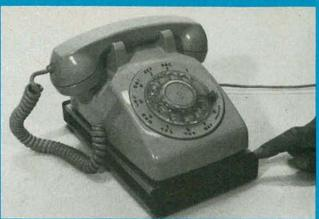
FIG. 6—ALTHOUGH SMALL ENOUGH TO FIT under a telephone, you don't need one to use the SmartModem from D.C. Hayes; all dialing is done from the computer or terminal keyboard.
