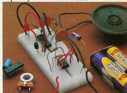
With your first module you'll receive this professional solderless breadboarding system. It enables you to connect components and build electronic circuits easily and quickly. It's used throughout the series and can be used later to design, build and test your own circuits.
