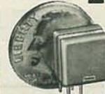
Just 1 1/32 x 3/8 x 1/4" SPDT contacts: 1 amp at 125VAC. 55-ohm, 90 mA coil. .100" centers. 275-240 ... 2.49
