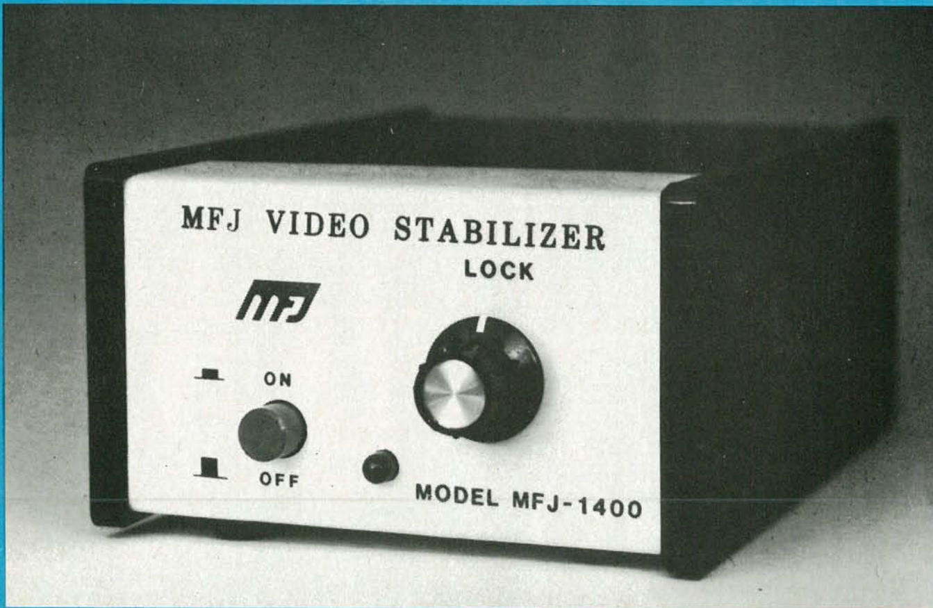
NEARLY ALL of the sync stabilizers on the market, including the one from MFJ enterprises shown above, reshape the vertical sync interval.
