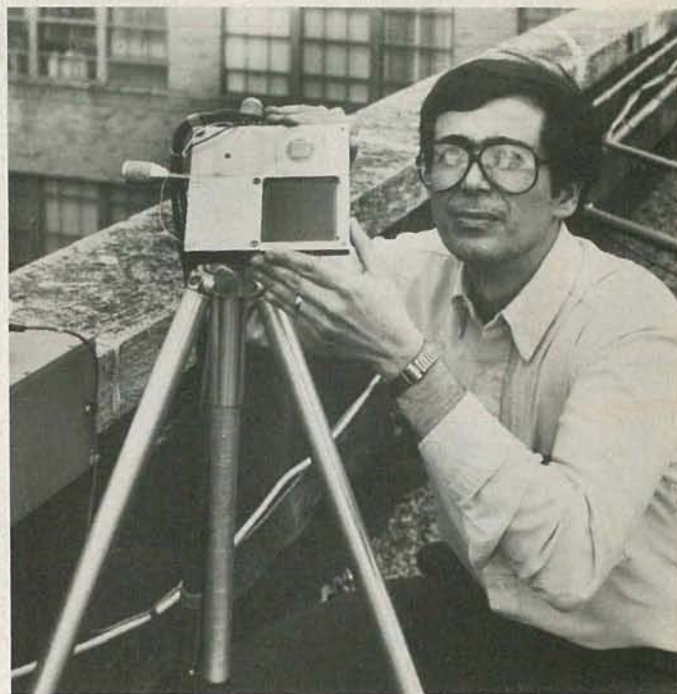
EFFICIENCY OF AMORPHOUS SILICON SOLAR CELLS is measured by Anthony W. Catalano, of the RCA Labs technical staff. The new higher-efficiency cells may open the way to large-scale production of solar power at costs competitive with the present oil-fired generating plants.
