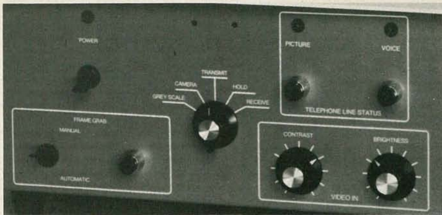
FIG. 21—PICTURE PHONE'S front-panel controls. The FRAME GRAB button is below and to the left of the five-position MODE switch.
