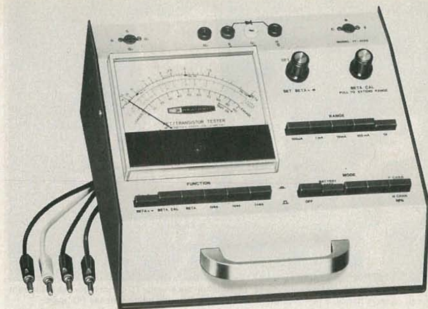
A TRANSISTOR TESTER, such as the one from Heathkit shown here, should be used to check all surplus and salvaged transistors before use.
