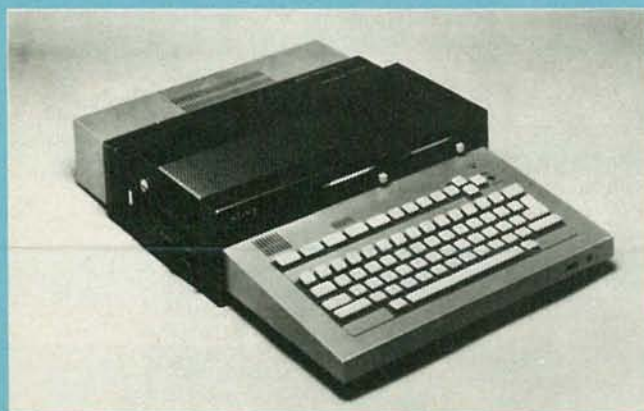
THE SMC-70 from Sony is supplied with 64K of RAM memory. It is shown here with optional 3.5-inch disk drives and RS-232C interface.
