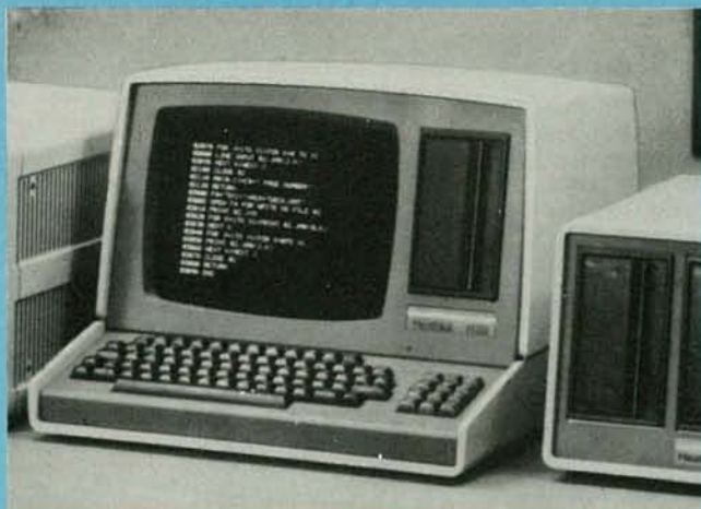
THE ZENITH Z90 is an upgrade of the Z89. The terminal-type housing looks identical for both computers.
