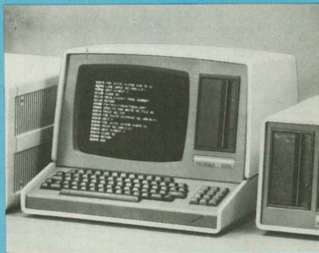
The H89 FROM HEATH is one of the few computers available in kit form. It is also available fully assembled as the Z89 from Zenith.
