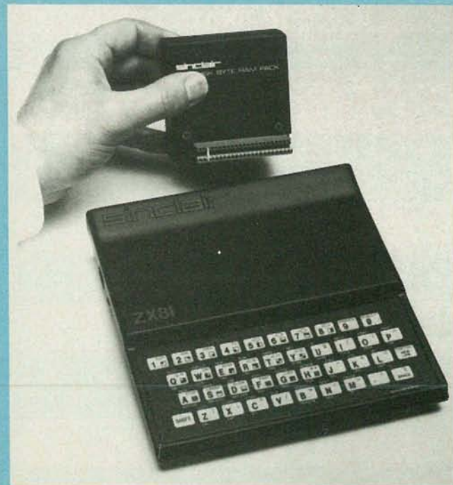
THE MEMORY CAPACITY, and the sophistication, of the Sinclair ZX81 can be increased by adding a 16K memory-expansion module.
