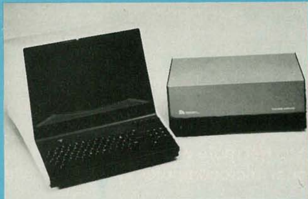
IN ITS NEARLY FULLY CONFIGURED FORM, the Netronics Explorer 85 includes a floppy-disk drive and CP/M.
