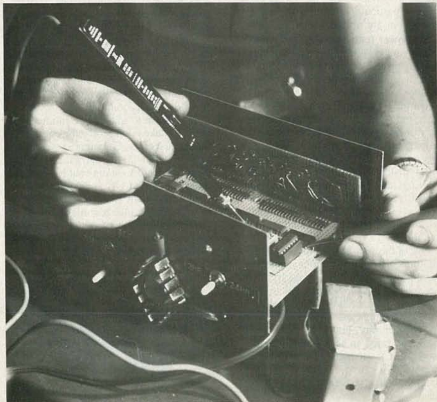
A MULTI-FUNCTION TEST PROBE, such as the one shown here, is handy for finding good components in surplus or salvaged equipment.
