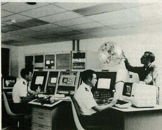
AIR FORCE TECHNICIANS TRACK SATELLITES at the ground-based Electro-Optical Deep Space Surveillance System facility in New Mexico. It is the first of five world-wide stations that will keep track of all man-made satellites in orbit within a range of 22,000 miles.
