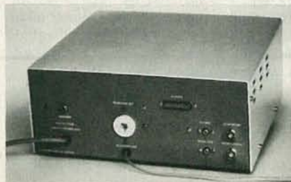
REAR PANEL of Picture Phone. Circuit-breaker reset is located above line cord at left.
