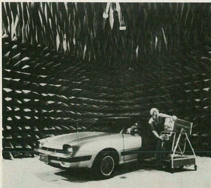
THE ABSORBING WEDGES, CONES, OR PYRAMIDS in this room make it look exactly like an acoustic anechoic chamber. Actually the cones are made of material designed to be especially absorptive to radio waves in the range of 14 kHz to 1 GHz. The chamber was installed by the Ray-Proof Division of Keene Corp. of Norwalk, CT.
