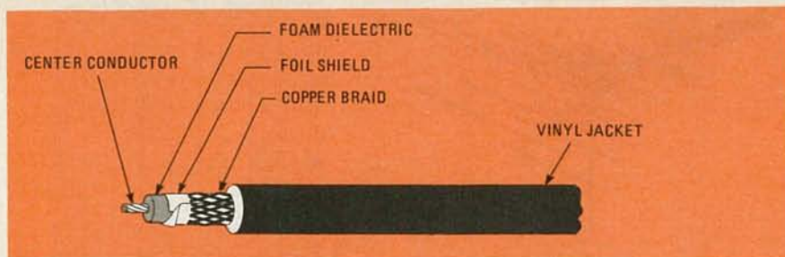
FIG. 14—FOR MAXIMUM SHIELDING AND DURABILITY, this type of coaxial cable should be used.
