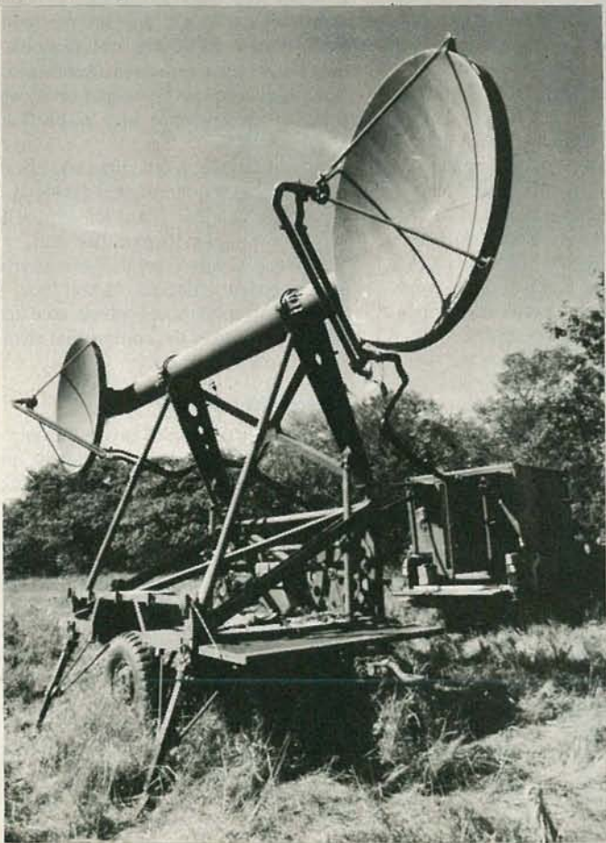
THESE PARABOLIC TROPOSCATTER DISHES are precisely aligned to scatter signals through the atmosphere to receivers up to 100 miles away.
