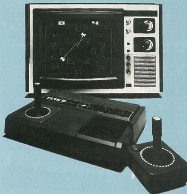
TANK II , one of the first non-programmable videogames from Atari. Note that the hand controllers closely resemble those used in the VCS.
