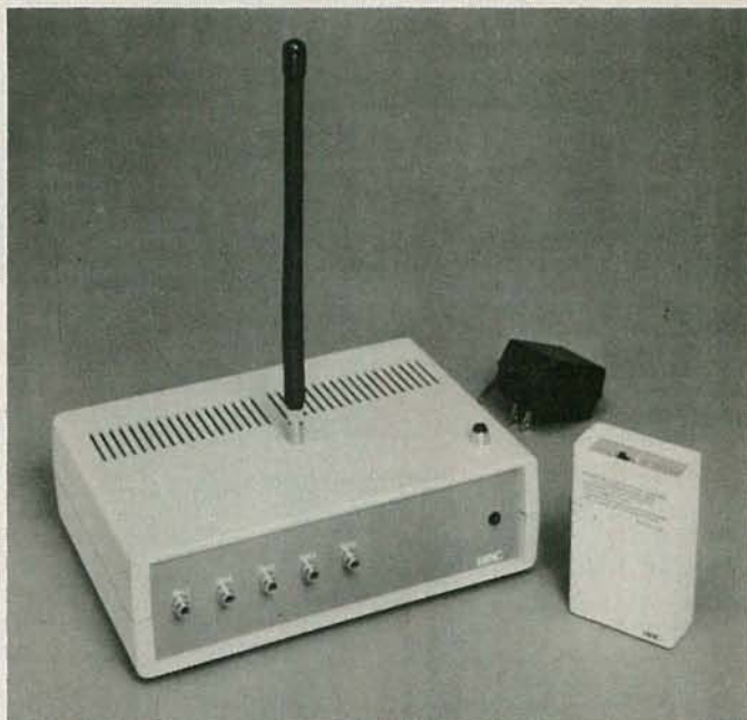
THE TACTILE COMMUNICATOR, with which the deaf or blind may receive signals they could not otherwise see or hear, at left; the pocket receiver at right.
