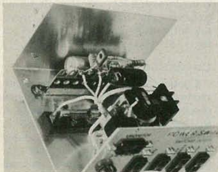
FIG. 3—THIS PARTICULAR VERSION of power switcher did not require 3-wire line cord, but yours probably will. Make sure that the ground wire makes good contact with case.
