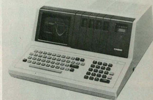
THE CASIO FX-9000P personal computer. The basic unit comes with a 4K RAM, a 5.5-inch built-in CRT, very extensive high-resolution graphics, and powerful mathematical functions for scientific, engineering and statistical operations.
