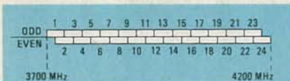
FIG. 4—HOW TO FIT 24 channels in a 12-channel bandwidth. Adjacent channels are overlapped, and odd-numbered channels vertically polarized; even-numbered ones horizontally polarized.
