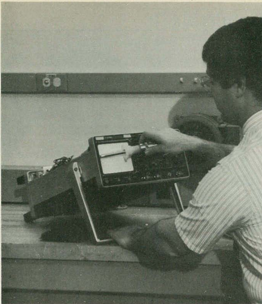
FIG. 2—A PIECE OF EQUIPMENT will not meet the UL Standard if any part that could give an electric shock is accessible to the user. Here, a UL technician is examining an oscilloscope for a potential shock hazard.
