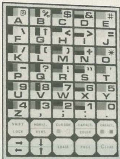
FIG. 10—KEYPAD LABEL shows many functions available. Function keys are pressed once to switch functions. Pressing them again returns you to original mode of operation.
