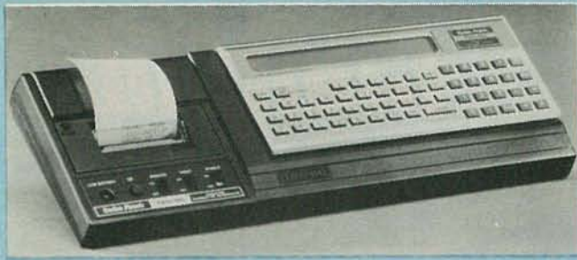
FIG. 1—THE TRS-80 POCKET COMPUTER is shown here with the slide-in printer and cassette interface. That peripheral turns the pocket computer into a complete "mini-system."
