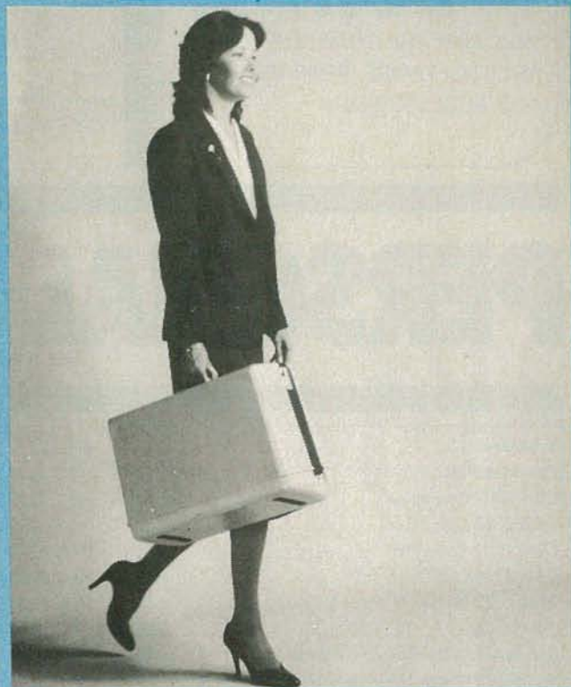
FIG. 1—A TRULY PORTABLE, all-in-one computer system the Osborne 1 folds up like a small suitcase so that it can be easily transported.
