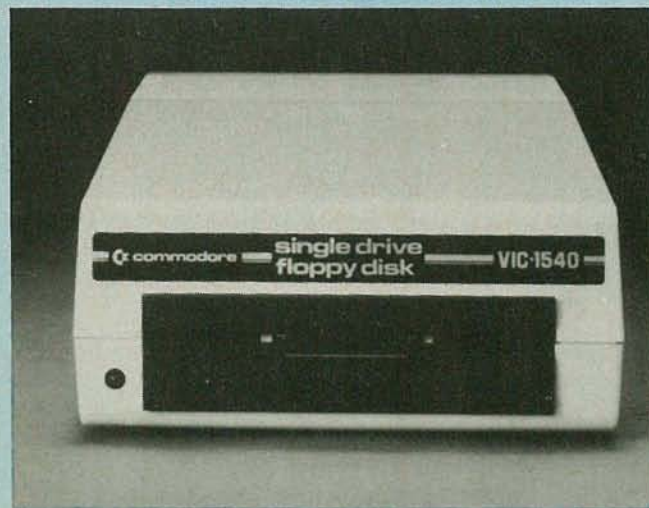
FIG. 2—FOR THOSE WHO PREFER a disk-based mass storage system, Commodore manufactures the VIC 1540 single 5¼-inch floppy disk drive.
