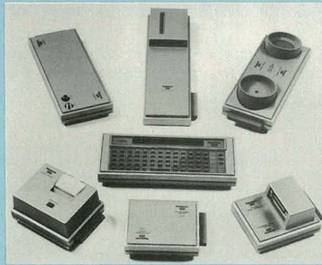
FIG. 3—SOME OF THE PERIPHERALS available for the Panasonic HHC pocket computer, as well as the device itself, are shown here. Among them are an RS-232 interface, a modem, a color-TV interface, and a small printer.
