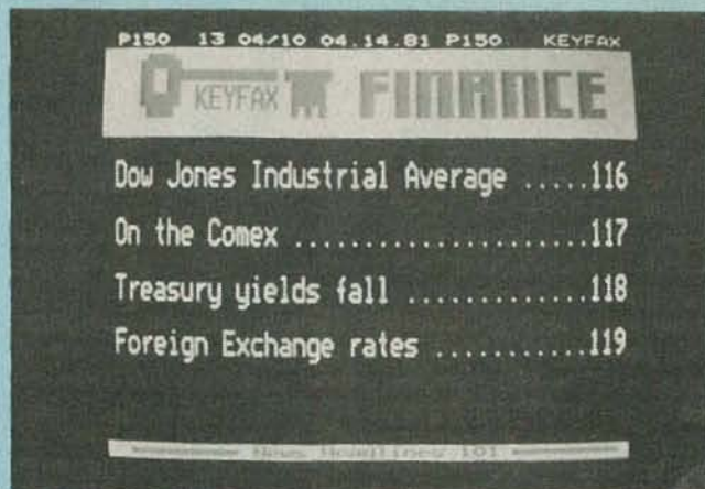
FIG. 4—A TYPICAL VIDEOTEX menu. The one shown here lists financial news stories. To call up one of them, the appropriate code is keyed into the accompanying controller.
