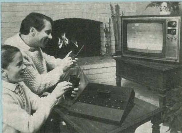
FIG. 1—THIS REMOTE-CONTROLLED Atari Video Computer System eliminates the controller wires and lets you control the action from anywhere in the room.
