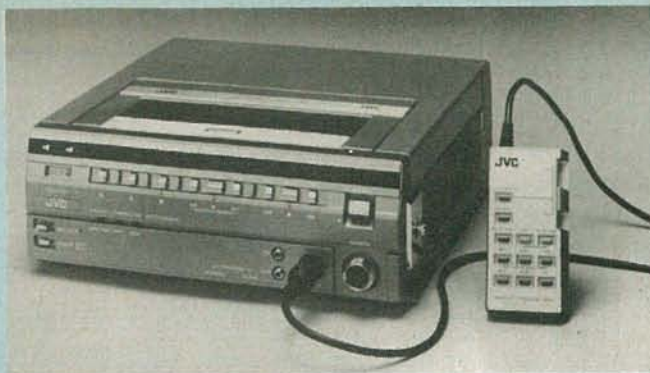
FIG. 11—JVC's HR-2200U has an edit-start control to eliminate noise or gaps between scenes.
