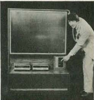
THE 50-INCH SYLVANIA SUPER SCREEN television system uses black matrix screen, which offers sharply improved contrast and bright lighting conditions.
