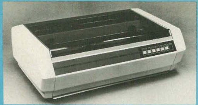
FIG. 1—THE MODEL IPS 5000A FROM DATAROYAL is a dot-matrix printer with a 120 cps print speed and a tractor-type paper feed.
