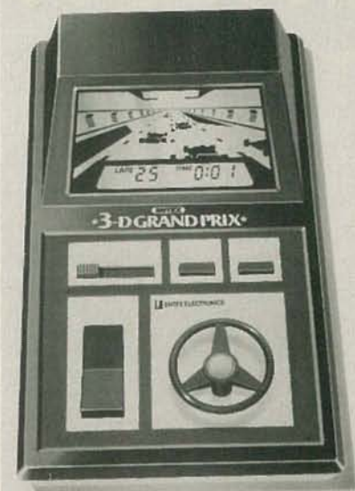
FIG. 2—LCD's CAN BE USED for graphics, as in Entex's 3-D Grand Prix game, but the displays are "hard wired" and cannot be changed by the user.
