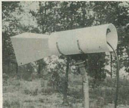
FIG. 30—THE LNA/FEED-HORN ASSEMBLY can be mounted inside a length of PVC pipe as shown here.
