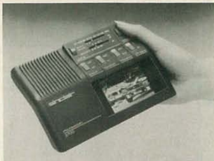
FIG. 15—SINCLAIR RESEARCH'S FLAT-CRT TV. The 6 × 4 × 1-inch unit is expected to sell in the $100 range when it is introduced in 1982.
