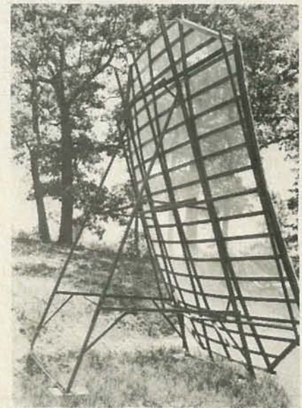
FIG. 22—REAR VIEW of the 12-foot 8-Ball antenna. All of the rear-support members are clearly visible.
