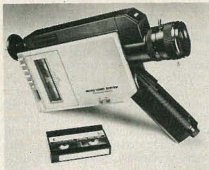
FIG. 4—INTEGRATED CAMERA/VCR unit weighs just 4.2 pounds. The cassette is about the same size as a standard audio cassette.
