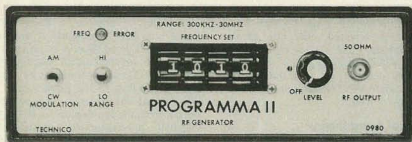
FRONT PANEL of the completed Programma-2 synthesized RF generator. Its layout gives the unit a professional appearance.
