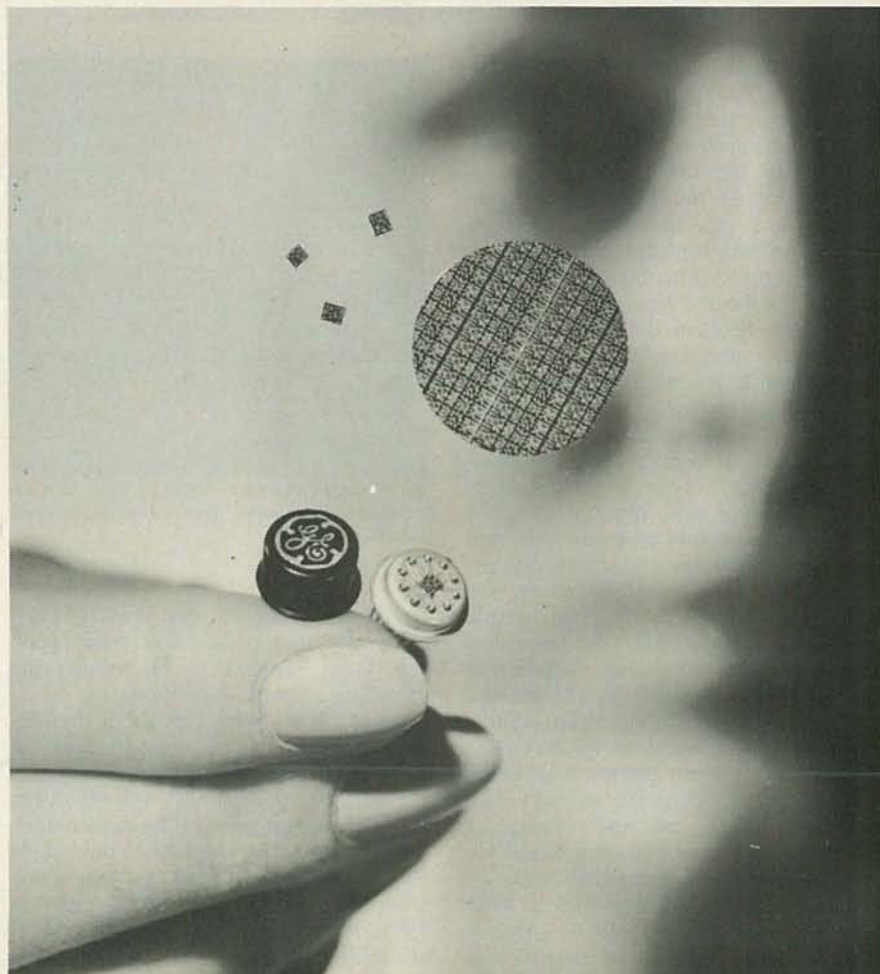
THESE EARLY (1962) IC's from General Electric contained as many as 18 transistors and 66 tapped resistors. Contrast that with the component count of modern VLSI IC's.
