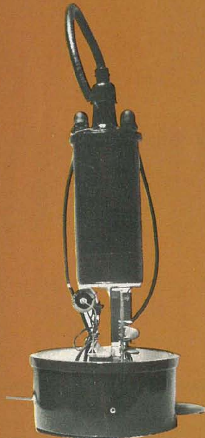
FIG. 4—A RIGHT-ANGLE BRACKET is epoxied to the top of transformer T1. The circuit board is mounted on the bracket using 1/4-inch plastic stand-offs. The connections to the ignition coil, and the lead from the coil's high-voltage terminal, will be concealed by the PVC pipe in the completed project.
