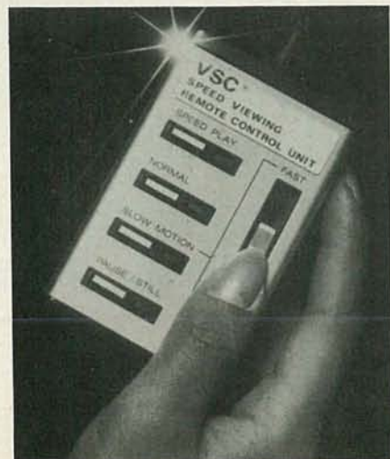
SPECIAL SPEED-VIEWING CIRCUITRY permits viewer to listen to sound while he scans the tape. The circuitry is in the VCR.
