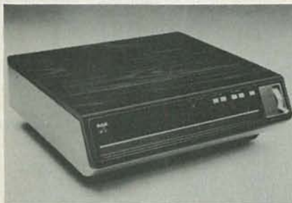
RCA VIDEODISC PLAYER. Disc is inserted, in its case, into the player. Your hand never touches it.
