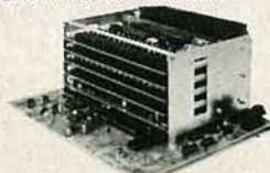
Explorer/85 With Level "C" Card Cage.
