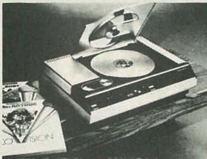
MAGNAVISON PLAYER WITH the lid up. The unit cannot be turned on until the lid is closed.
