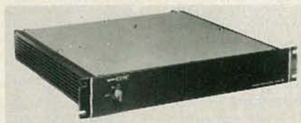
FIG. 1—MONAURAL power amplifier, the model TA-N-900 from Sony does not use negative feedback.
