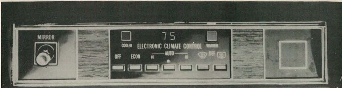
ELECTRONIC CLIMATE CONTROL offered on the 1981 Cadillac provides heat and air conditioning automatically. It features a digital temperature readout.
