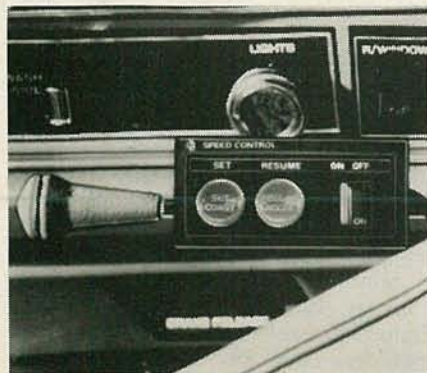
FIG. 4—CRUISE CONTROL from Sears mounts on the dash or on the turn signal stalk.
