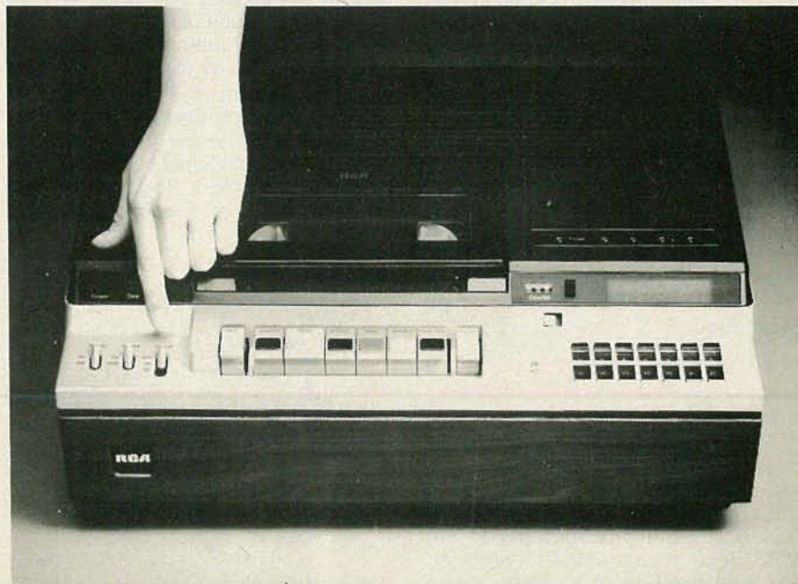
THE RCA model VDT600 VCR uses the VHS system and has three selectable speeds.
