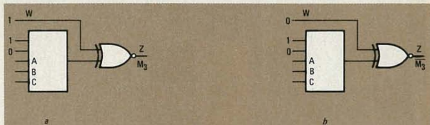
FIG. 4—TYING ONE OF THE five inputs high and one low leaves a 3-input majority-logic gate.
