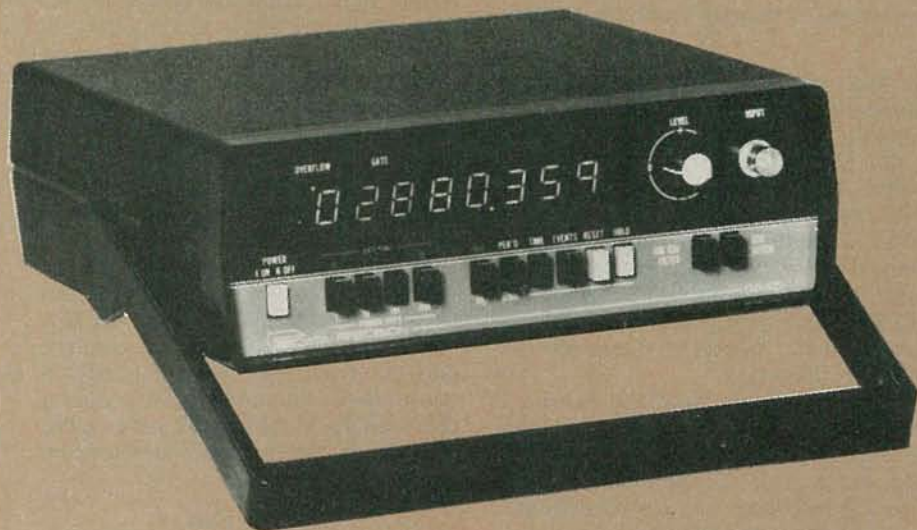
DATA PRECISION MODEL 5845 (above) has a pulse-resolution of 15 nS. Low-pass filter maximizes noise-rejection when working with low frequencies.
