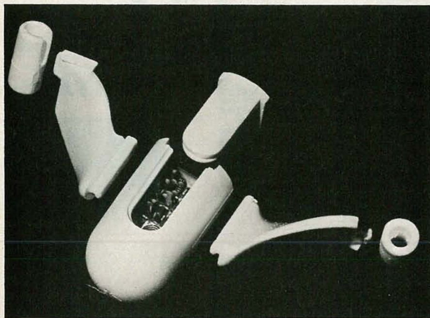
THE AIRSONDE BODY, body door, wings and wing tubes, and the tongue-and-groove method of connecting them together.
