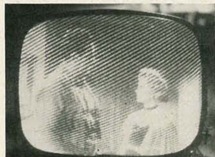
FIG. 7—FM TRANSMITTERS in police cars may cause occasional interference.
