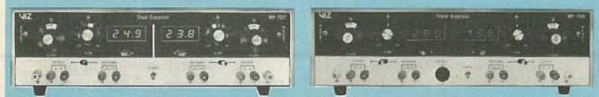
Dual, Two 0-25VDC, 0-2A supplies (0-50VDC in series). Two voltmeters 0-99.9VDC. WP-707 $299 Triple, Two 0-20VDC, 0-2A supplies (0-40VDC in series). One 5VDC (0-4A) fixed supply. Two voltmeters 0-99.9VDC. WP-708 $333
