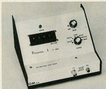
FIG. 7—THIS LAYOUT works well, but is not ideal. Output jacks and "level" pot should be located closer to one another to keep leads short.
