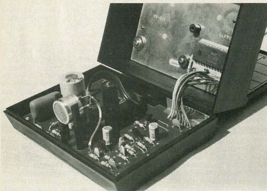
FIG. 3—CONTROLLER MODULE, despite its complexity, is surprisingly small—only 4\frac{1}{2} \times 3\frac{1}{2} \times 2\frac{1}{2} inches.
