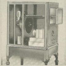
JENKINS PROJECTION RADIOVISOR, developed in 1931, used deForest's new neon-crater tube and a 1-inch scanning disc with sixty ½-inch lenses to throw a flying-spot image on the rear of the ground-glass viewing screen.
