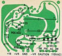
FIG. 4—POWER-SUPPLY PARTS-PLACEMENT
