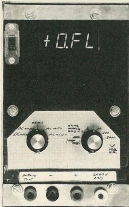
FIG. 3—THIS DISPLAY on the readout can not be mistaken for anything other than overflow.
