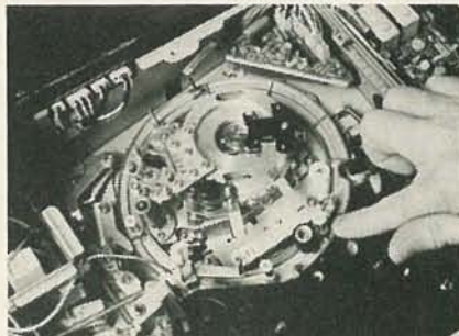
THREADING THE TAPE begins when the threading ring revolves counter clockwise.
