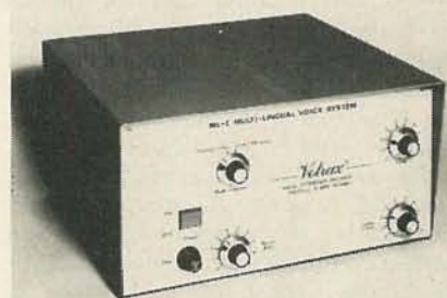
MULTI-LINGUAL VOICE SYSTEM, model ML-1, also from Votrax, speaks in seven languages, including Farci.
