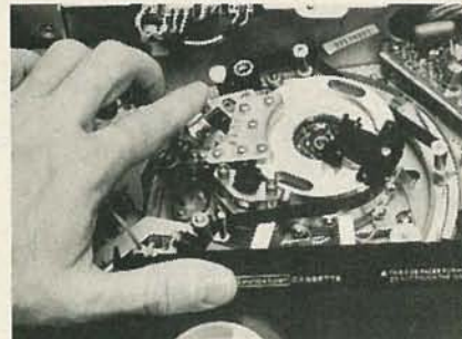
THE THREADING RING continues to revolve wrapping the tape closely around the face of the video-head drum.
