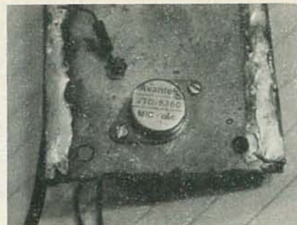
THIS INNOCENT-LOOKING DEVICE is capable of producing +10 dBm of local oscillator signal at 4 GHz! Avantek VTO 8360 is a microwave oscillator device totally self contained. It mounts on full-foil side of board with pins (leads) accessible on opposite board side with active 4-GHz circuits.
