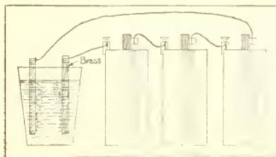
How Wires are Connected
