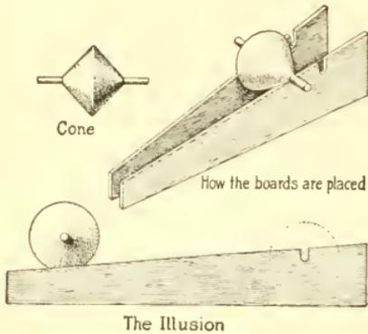
one end will be higher than the other by a little less than half the diameter of the cone. Thus it will be seen that the diameter of the cone determines the length of the slope of the tracks. A notch should be cut in the tracks, as indicated, for the shaft to drop into at the end of the course.
