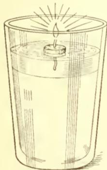
be of such a length as to dip into the oil, but not long enough to reach the water. The upper surface of the cork may be protected from the flame with a small piece of tin bent over the edges
