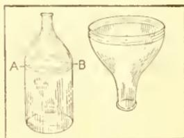
sene around the outside at A and B as shown in the sketch. Light the string and allow it to burn until the glass is heated, then plunge the bottle quickly into water. The top or neck will then come off easily. The sharp edges are ground or filed off smooth. This will make a good emergency funnel which serves the purpose well for filling wide necked bottles.—Contributed by Jos. W. Sorenson, Everett, Wash.
