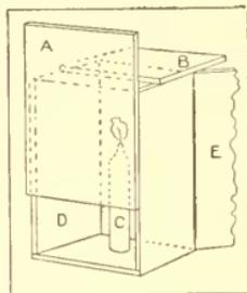
Remove the bottom of the box, and nail it in position as shown at A. Remove one end, and replace as shown at B.
