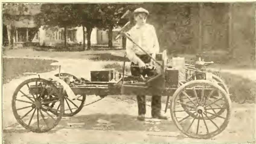
Side View: Seat Removed to Show Construction
