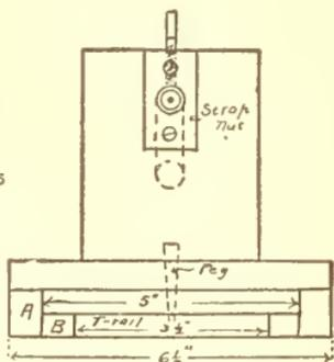
ter, using longer 3/16-in. stove bolts with heads countersunk. Rotate the lathe, and with a gimlet bore a hole at the exact center and through the board. Now take off the board and countersink on the back a place for the head of a coarse threaded screw. Turn in a 1 3/4-in. screw, replace the board and any block held on the end of the rotating screw will turn on and be held while being turned.—Contributed by L. L. Winans, Mexico, Mo.
