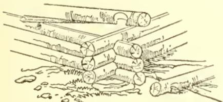
How the Logs Lock at the Corners
