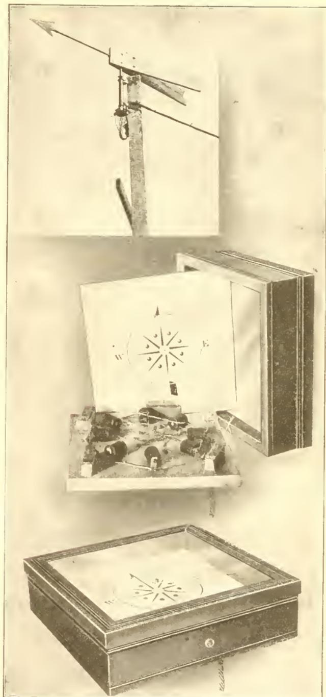
The Wind Vane, Magnets and Indicator
