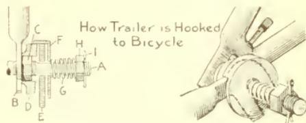
Fig. 2—The Hook in Position
