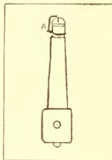
Take any small piece of wire about 2 in. long and twist it around a gas-burner as shown at A in the sketch. Have the tip of the burner about  $\frac{1}{8}$  in. below the end of the wire. The wire must be just far enough away from the center of the burner to keep it out of the flame, or else it will melt.
