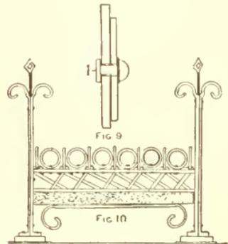
for making these stands, as every part is bent as described in connection with the bending forms, and the portions are simply riveted at the different junctures. Both iron and copper rivets are used as at I, in Fig. 9, a cross sectional view.
