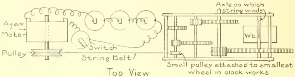
6 in. wide and 12 in. long. Remove the mainspring from the clockwork and make a small pulley and fasten it on the axle of the smallest wheel in the mechanism.
