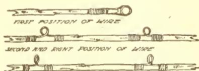
Fig. 3—Method of Making a Trout Rod
