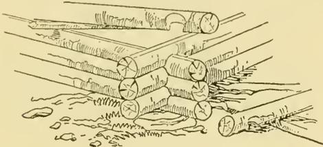
How the Logs Lock at the Corners
