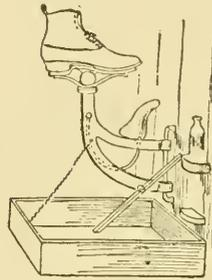
This cabinet folds to the wall and projects only about 2 in. into the room. When dropped down a chain pulls the foot rest into position and a hinged arm supports the box underneath to catch all dust which may drop from the shoe. A shoe form may be provided, also, for polishing shoes when not on the feet.
