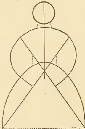
strings or thread, and the other lines indicate the kite sticks. Be careful with your measurements so that each side of the kite corresponds exactly and is well balanced. Also see that every point where the sticks intersect is firmly tacked and bound.
