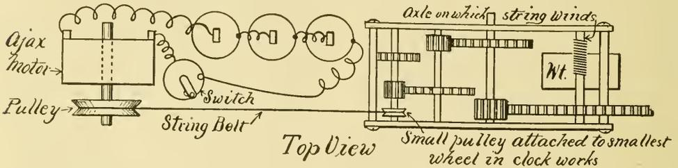
The materials necessary are a small battery motor, three or four cells of batteries, an old clockwork, and a board about 12 in. long and 6 in. wide. Remove the main-spring from the clockwork and make a small pulley and fasten it on the axle of the smallest wheel in the mechanism.
