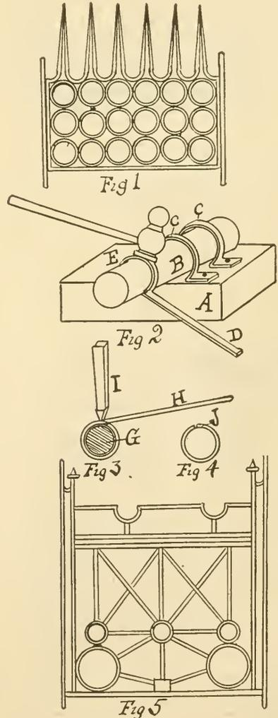
Fig. 1 is a design of grate front used for various purposes in connection with grate fires. The series of rings are united by a rivet between each at the joining point. With thin metal the holes can be punched
