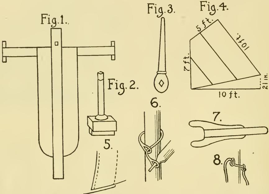
an inch and a half at the top. This fits in the square hole, Fig. 1. The horn should be 5½ feet long, 2x3 at the butt and 1 inch at the end.
