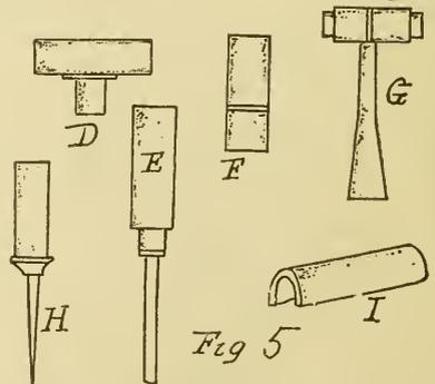
etc. G is a mallet-like tool, with the tube portion sustaining the wood or lead plugs for "soft" work. H is a prick tool made
