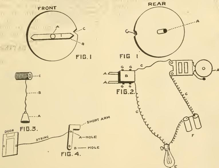
nail it securely to the round piece. At A make a hole large enough to run a 20-penny nail through.
