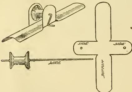
Fig. 4.—Method of Making the Reel
