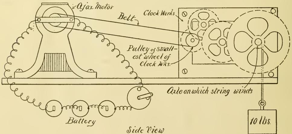
string belt. Now fasten a piece of strong cord or chalkline to the axle of the large wheel of the clockwork and put a weight of about 10 or 12 lb. on the end of the string.
