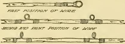
Fig. 3.—Method of Making a Trout Rod
