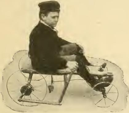
working wooden "driving rod," connected to an iron crank fastened to one rear wheel, succeeded in producing a machine that makes quite good speed. The illustration shows the arrangement, which any bright boy can make with a few tools. Earl made this wagon motor without any suggestions or assistance from anyone.
