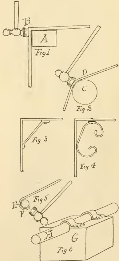
In some of the work required, it is necessary to shape a complete loop or circle at the end of the piece. This may be wrought out as in Fig. 5. The use of a bar of iron or steel is as shown. The bar is usually about 2 inches in diameter and several feet in length so that it will rest firmly on a base
