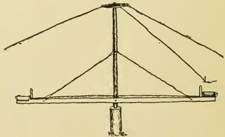
center pole should be 10 ft. high. An old wheel is mounted at the top of the pole, and the pole works in the wheel as an axle, says the American Boy. The wheel is anchored out by several guy wires. The seat arms may be any length desired. A passenger rides in each seat and the motor-man takes his station at the middle.
