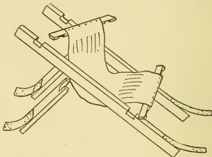
Fig. 3.—Folding Chair Sleigh.—Top Parts Disconnected
