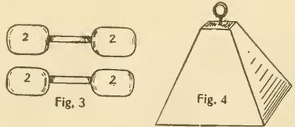
length of rod between (Fig. 2.) It is well to first string the two inner disks on the bar and then drive a few nails through each end of it before pushing into the cement, to give it a grip. The disks are then pushed along the rod to fit into the open end of each can. Put a wedge in each end of the can to hold the bar in place. The other dumb-bell is made in the same manner.
