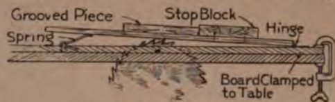
How to Groove Short Blocks
