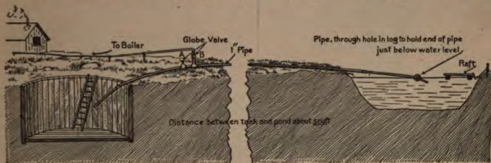
Filling Tank with a Siphon
