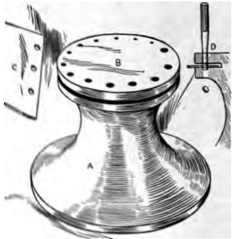
Punching Holes in Sheet Metal
