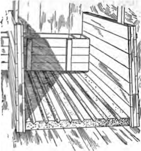
Cement Stall Floor
