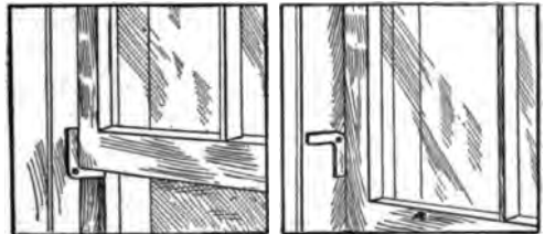
FIG. 1 Catch in and out of Position
