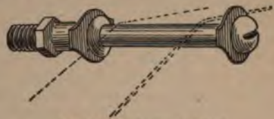
Idler Made of Bicycle Pedal
