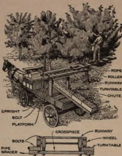
DETAIL OF RUNWAY LOCKING ARRANGEMENT With This Machine Two Men Are Able to Do the Work of Eight. Fruit may be Picked from Four Trees without Changing Its Location
