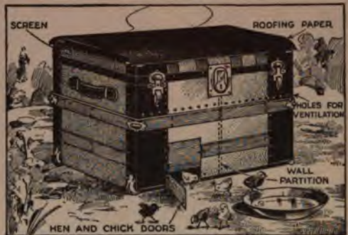
A Few Changes Turn an Old Trunk into a Two-Compartment Chicken Coop Which Lasts for Years
