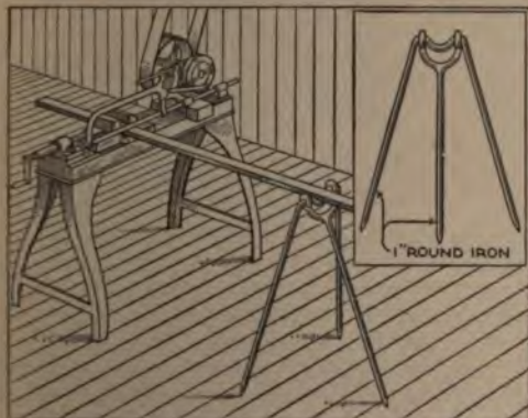
Stock Support for Power Hacksaw: The Height of the Tripod can be Varied by Changing the Spread of the Three Legs
