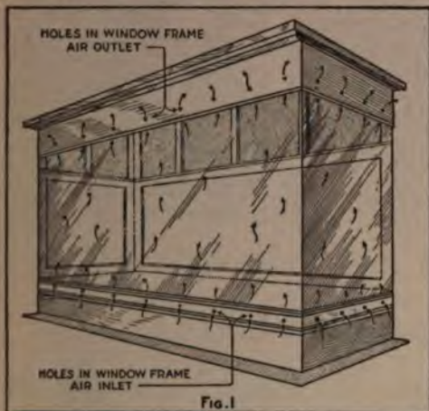
When the Window Glass is Set in a Wooden Frame Which Extends above the Window Floor, All the Holes Required may be Made in This Frame
