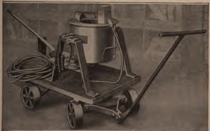
One-Hundred-Pound Standard Bench-Type Electric Pot Used for Melting Bearing Metal: The User Mounted This on the Small Truck So That the Metal in the Pot could be Carried Directly to the Work
