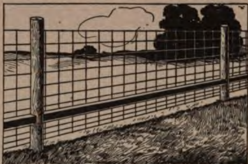
If the Posts are Braced against Each Other by Timbers Firmly Mortised In, the Fence is Strengthened against the Pull of the Wire
