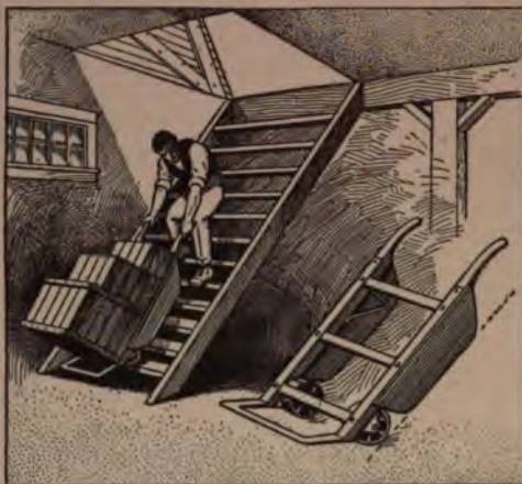
Difficulty in Moving a Hand Truck up or down a Stairway is Considerably Reduced by Providing Runners Back of the Wheels
