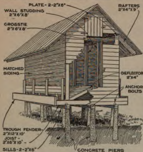
A Cattle Feeder That Is Particularly Useful for Feeding Cattle during the Winter, on Chopped Forage, or Grains: It Holds Approximately 500 Bushels of Feed
