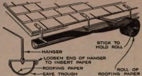
Eaves Troughs That are Beginning to Rust and Leak can be Satisfactorily Repaired by Lining Them with a Strip of Roofing Paper
