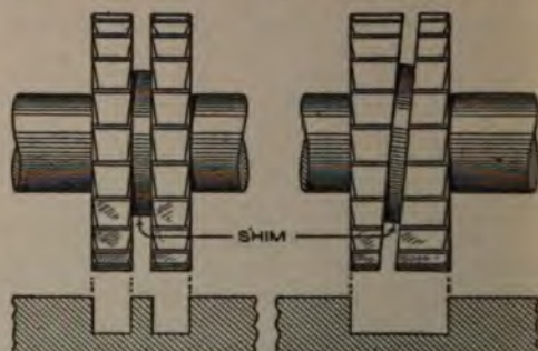
A Set of Two Milling Cutters, Ground to an Angle and Shimmed Apart, will Produce Finished Slots, of Variable Width
