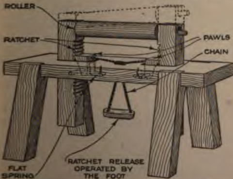
A Wooden Horse for Wood Shops That Has Some Valuable Features: The Height and Position of the Roller Are Instantly Adjustable
