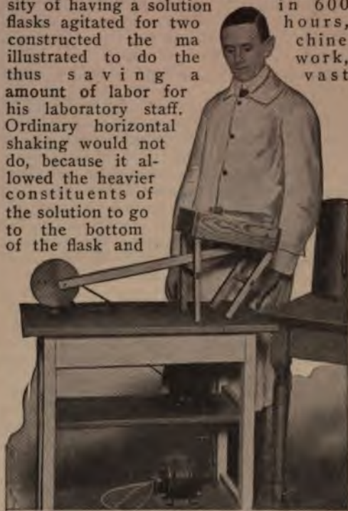
A Machine Built by a Bacteriologist Agitates a Solution with a Motion Approximating That of the Hand in Shaking It
