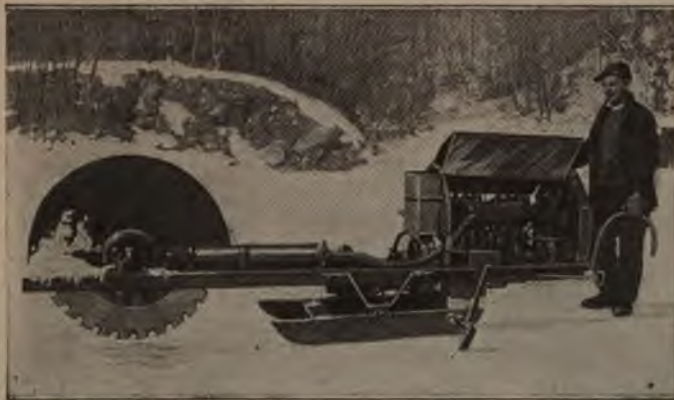
Automobile Parts are Used to Make a Self-Propelled Ice-Cutting Machine. At the End of the Season the Machine is Dismantled and the Car is Reassembled
