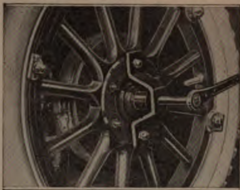
Pulling a Wheel from a Full-Floating Axle Is Easy When a Suitable Tool Is Applied; the Illustration Shows a Simple Tool for This Purpose
