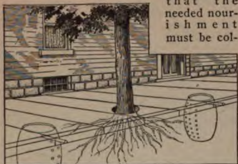
Barrels, 20 to 30 Feet Apart, are Buried beneath the Concrete Sidewalk to Act as Cisterns and Provide Artificial Irrigation
